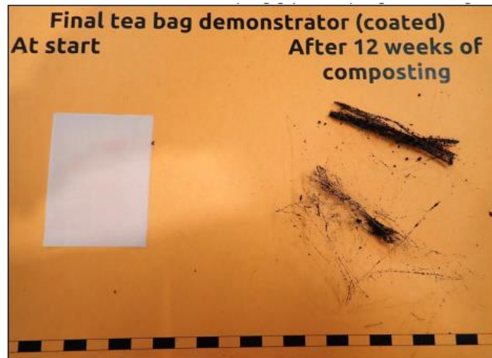
Fig. 4: Disintegration of the alginate-coated PLA-based tea bag after 12 weeks of home composting.
