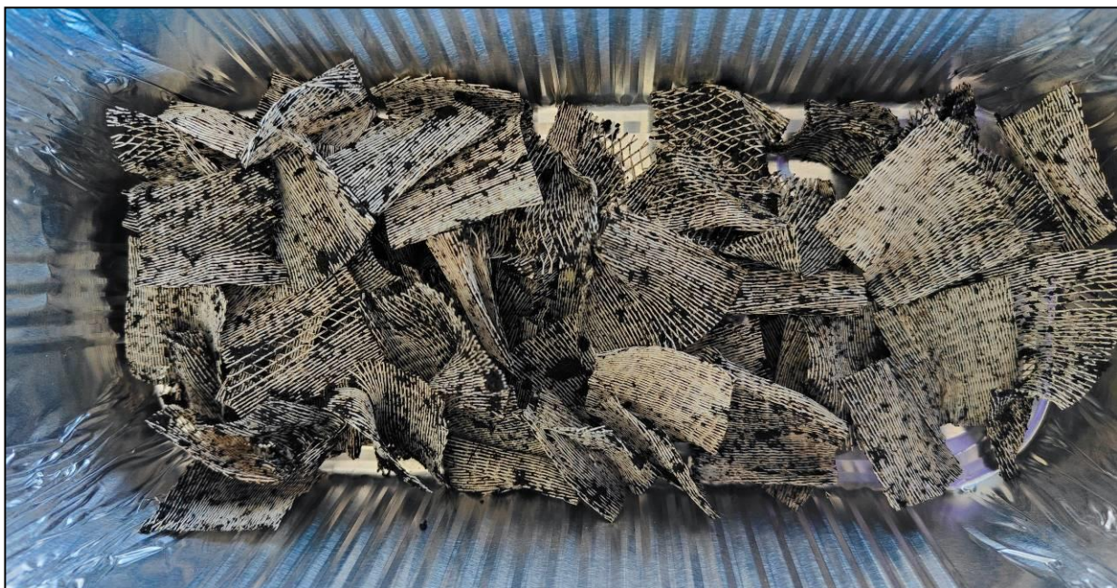
Figure 19: Visual representation of Oriented net after 56 days of dry, anaerobic mesophilic conditions
