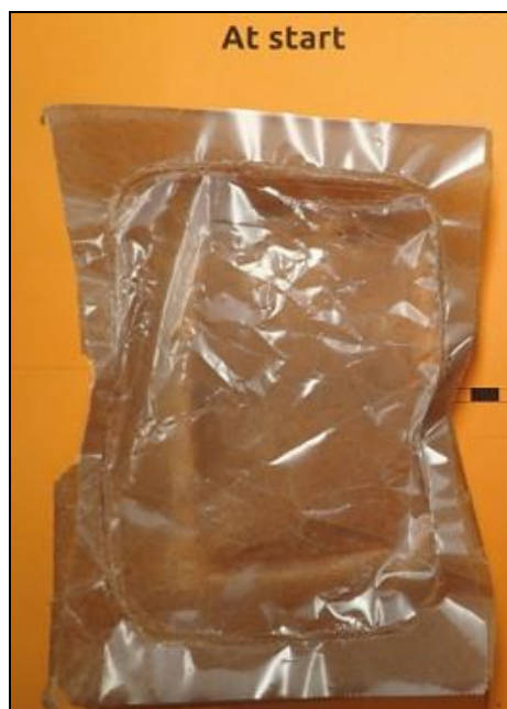
Figure 11: Visual presentation of complete tray with film (Tray Formula N1 Thermoformed and Thermosealed with Flexible Film Formula N2), in a thickness of \pm 0.05 mm (film), \pm 0.26 mm (bottom), \pm 0.39 mm (edge)
