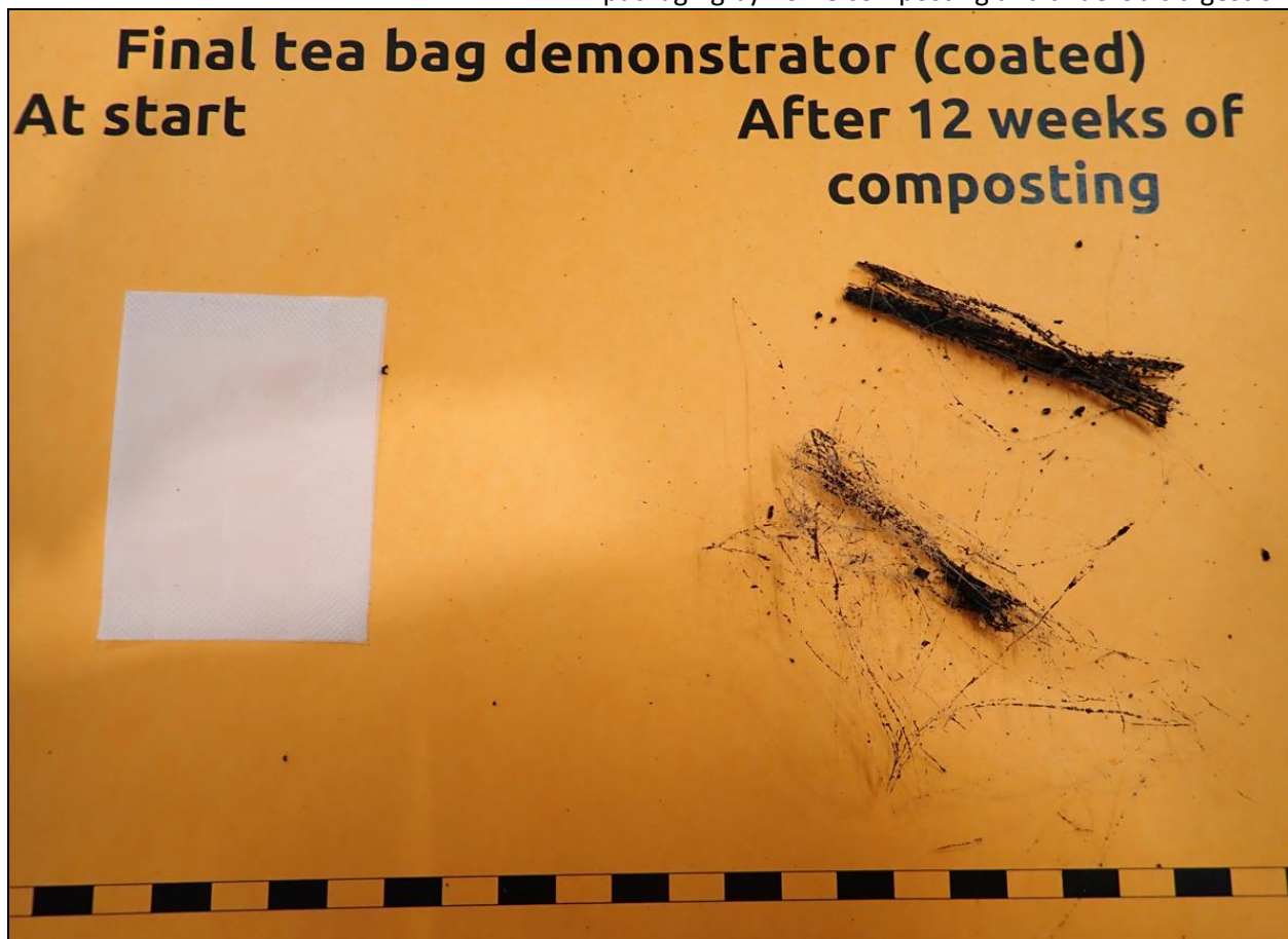
Figure 6: Visual presentation of the disintegration of alginate coated PLA-based tea bag after 12 weeks of home composting
