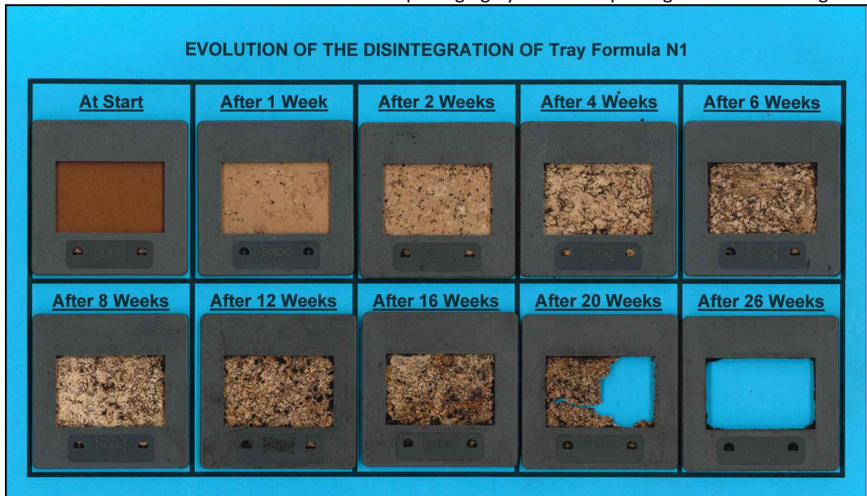
Figure 10: Visual presentation of the evolution of the disintegration of test material Tray Formula N1 in slide frames during the home composting process
