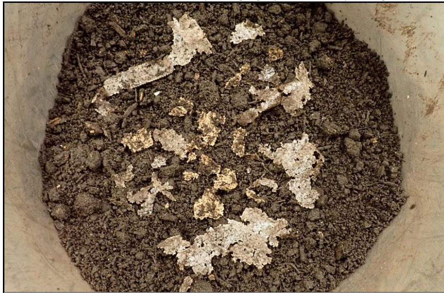
Figure 12: Visual presentation of the contents of a composting reactor with Tray Formula N1 Thermoformed and Thermosealed with Flexible Film Formula N2, added as such, after 10 weeks of composting at ambient temperature
